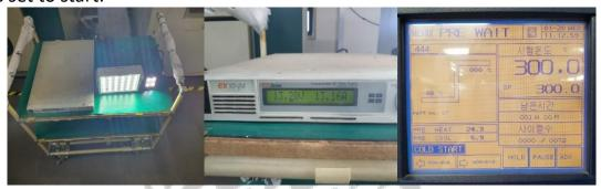
3. Leave the item at minus 60 degrees Celsius for an hour and check whether the item lights up as a pre-test. Start the main test, leave the item for 24 hours at minus 60 degrees Celsius.
