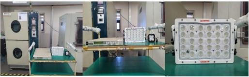
2. Set DC power supply 13.2V, and check every equipment is working & set well. Test is set to start.
